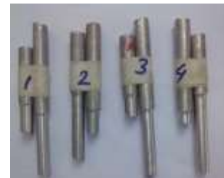
Fig.6 Tested tensile samples
